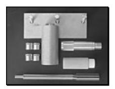
A4LD Lever Bore Repair Tool Kit - #OM-140T Fixture Plate, 7/8" Reamer, Bushing driver, 5 Solid Bronze Bushings, Cutting Solution Concentrate
