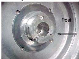
**Problem:** This post supports a sealing ring sleeve. The center of the post holds a bushing that tends to ruin the case when it fails. Getting the bushing out is difficult.
