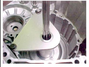
Bolt on the top plate to center and stabilize the reamer guide. Use WD-40 to lubricate the reamer. Use a 1/2" drill on slow speed and press firmly until it stops cutting. There is a definite change in the feed when it bottoms out. Carefully extract the reamer. Store it in the plastic case to keep it sharp.
