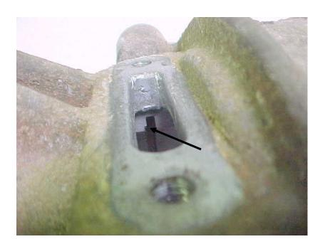
The extension housing bearing snap ring wears into the case causing the rear bearing to walk back and forth in the case.
