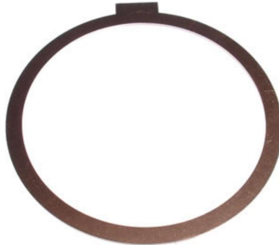
**Omega Machine & Tool has come out with a steel washer/spacer to repair the 48RE rear extension housings. The snap ring wears into the case allowing the geartrain to move back and forth. This ring saves the housing by positioning the rear bearing where it belongs.**
