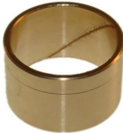
**The forward drum bushing carries a lot of load in this transmission. We've made a one piece bushing for better support and ease of installation.**
