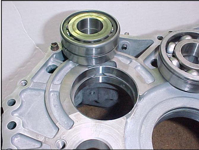
Many of the different Honda cases are wearing the bearing pockets. This allows the gear-trains to run off center, resulting in increased noise and decreased transmission life.
