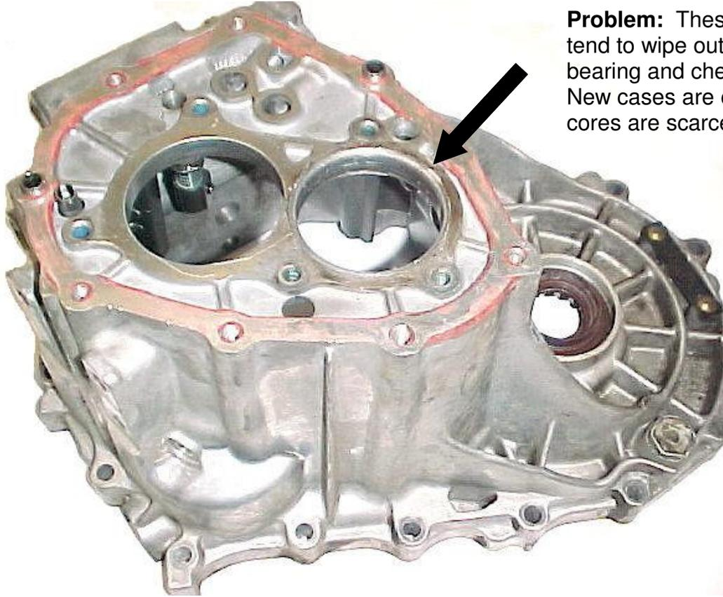
**Problem:** These Toyota cases tend to wipe out the countershaft bearing and chew up the case. New cases are expensive and cores are scarce.....
