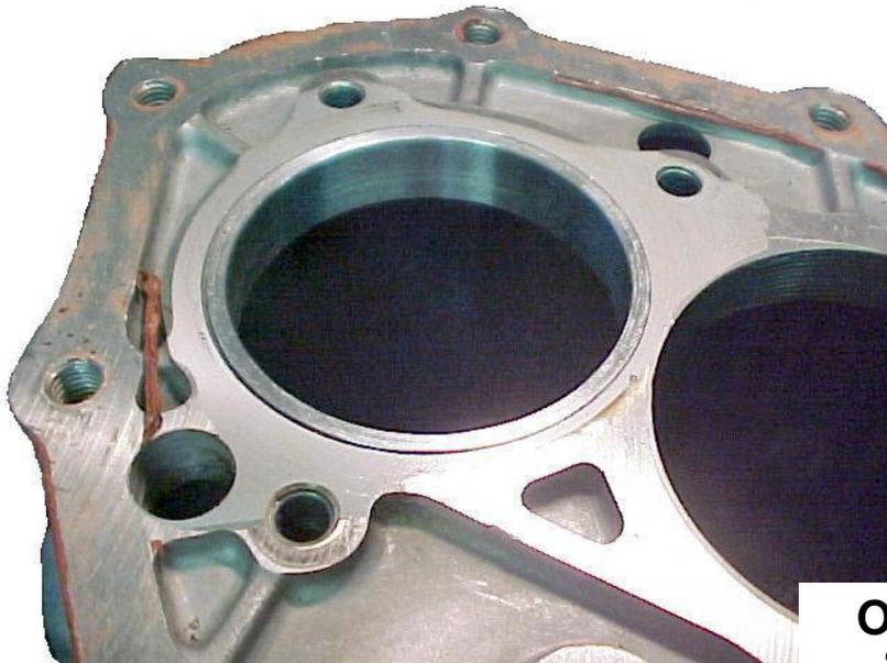
**Solution:** Omega's sleeve re-mounts the bearing back on its original bore location. The sleeve has a lip or "hat" that seats in a recess to keep the snap ring from pushing it back into the case.
