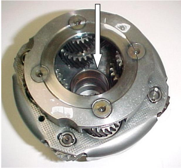
This planetary unit from a AW-5550-SN has a common flaw. The bushing closest to the sun gear is poorly supported and likes to spin in the cage.
