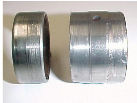
All is not lost. We bore out the cage to clean up the wear and also remove an unmachined shoulder between the bushings.
